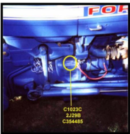
These are the most important numbers on the whole tractor. These are all someone needs to correctly ID a tractor as to when and what model it is.
