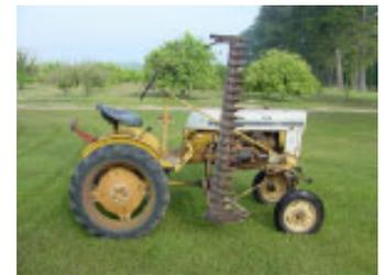
Figure 30. Sicklebar mower on small offset tractor.
