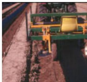
Figure 32. Plastic mulch layer on compact tractor.
