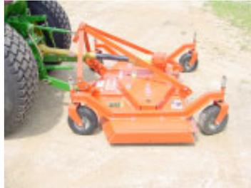
Figure 25. Heavy-duty finishing mower on compact tractor.
