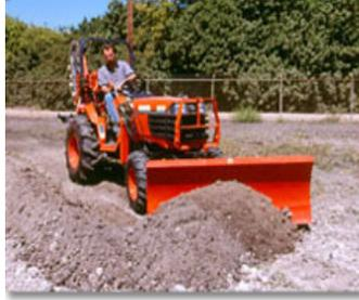
Figure 7. Front blade on compact tractor. (Photo from Kubota)
