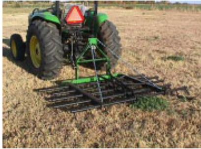
Figure 20. Spike-tooth harrow for compact tractor. (Photo from
