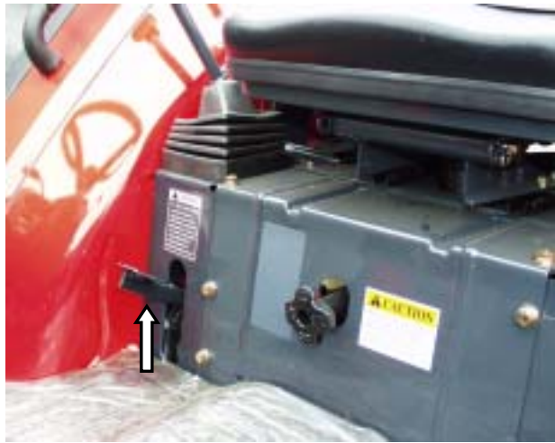
FIG.2-25 Diff-lock pedal
