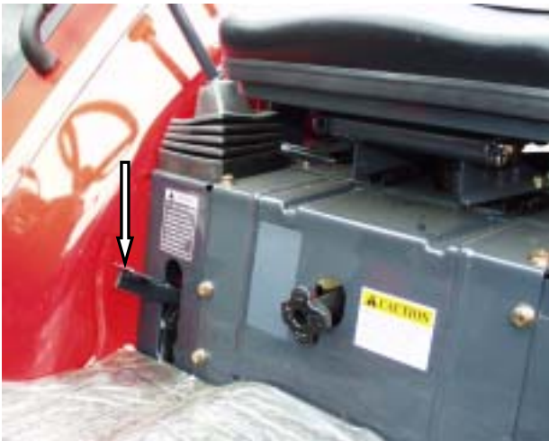
FIG.2-52 Diff-lock pedal
