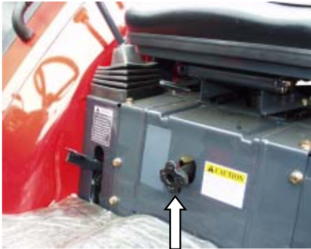
FIG.2-40 slow return check valve knob
