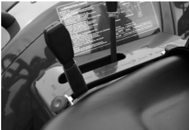
FIG.2-27 position control lever
