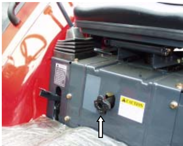
FIG.2-23 Slow return check valve
