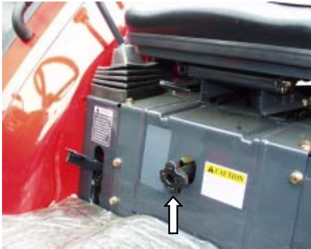
FIG.2-31 Slow return check valve
