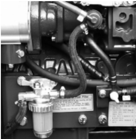
Fig.2-9 Fuel filter
