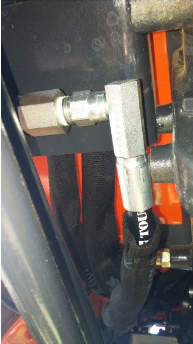
M18 x 1.5 to 1/2" NPT Adapter and 1/2" 90 deg NPT Swivel
