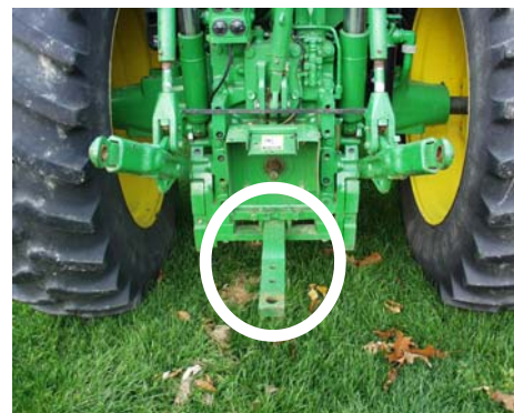
Figure 5.1.c. The tractor drawbar is the only safe place to connect a load. Do not hitch higher than the drawbar so all pulling forces stay below the tractor’s center of gravity. For most operations, the drawbar should be placed midpoint between the rear tires to maximize pulling power. Hillside operations may require a drawbar adjustment to one side to balance the pulling forces.
