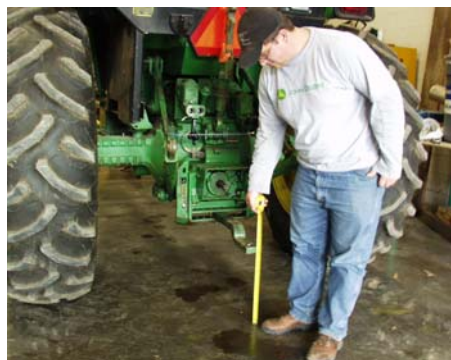
Figure 5.1.d. Tractor drawbars are designed at the correct height from the ground to keep the pull forces below the center of gravity. See Table 5.1.a. Only use the drawbar to tow a load. A swinging or floating drawbar permits adjustment of the center line of pull to be maintained even on a hillside.
