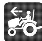
The tractor will travel at a constant speed without the need to continue pressing the accelerator/drive pedal.
