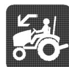
The travel speed will be automatically decreased to prevent engine stalling when the engine speed falls due to a load.
