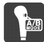
With each "A mode" and "B mode", one preset engine RPM and one maximum travel speed can be switched between with a single button press of the A/B switch (2).
