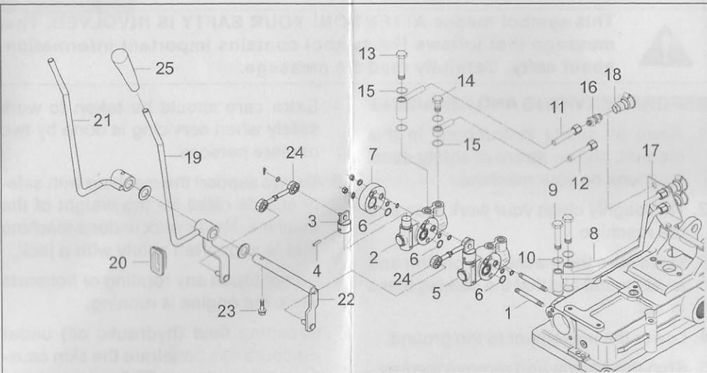
10. Install the longer studs (1). Be sure to apply the LOCTITE on the thread of studs.
