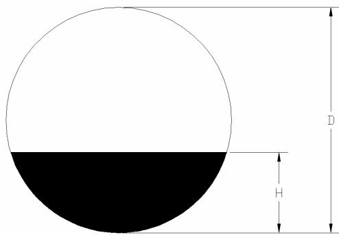
The Following equation can be used to calculate the number of gallons remaining in a horizontal tank if the height of the liquid remaining in the tank and the diameter of the tank are known.
