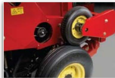
The drive even disengages automatically when the drill is raised, providing simple, trouble-free operation.
