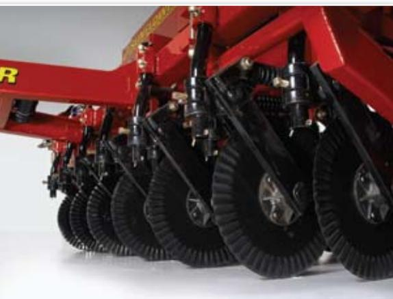
permit the wedge-shaped double-disc V openers to place seed directly into tilled soil for early germination.
