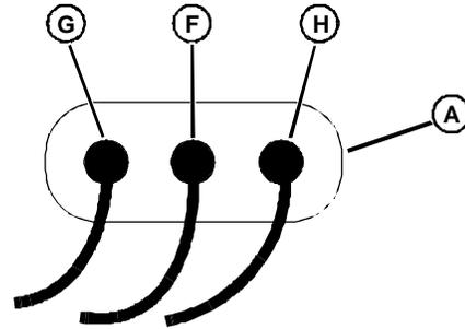
7. Connect voltmeter negative lead to air pressure sensor (A) black wire terminal (F). Connect meter positive lead to red/blu wire terminal (G). Measure input voltage. Voltage should be about 5 volts.
