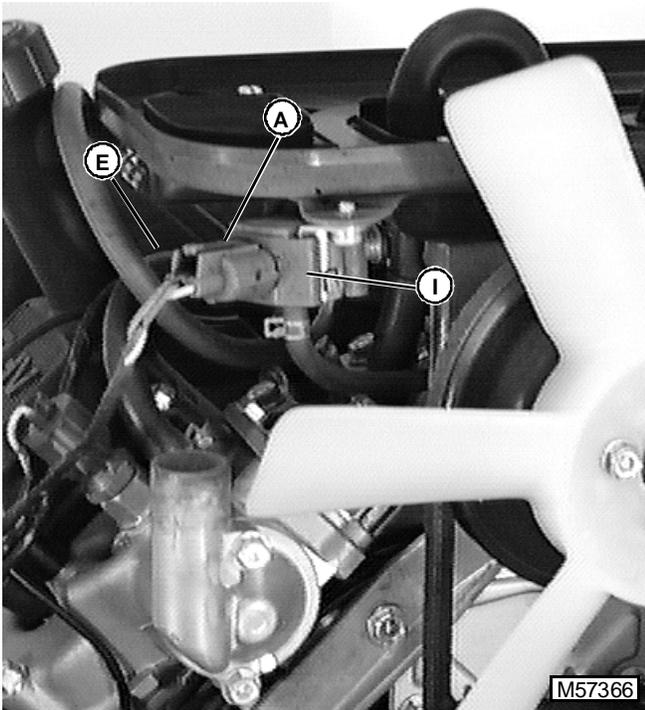
2. Disconnect air pressure sensor connector (A).
