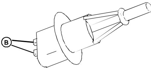
3. Measure resistance across air temperature sensor terminals (B).
