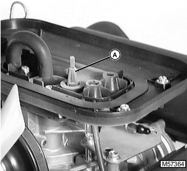
2. Disconnect air temperature sensor connector (A).
