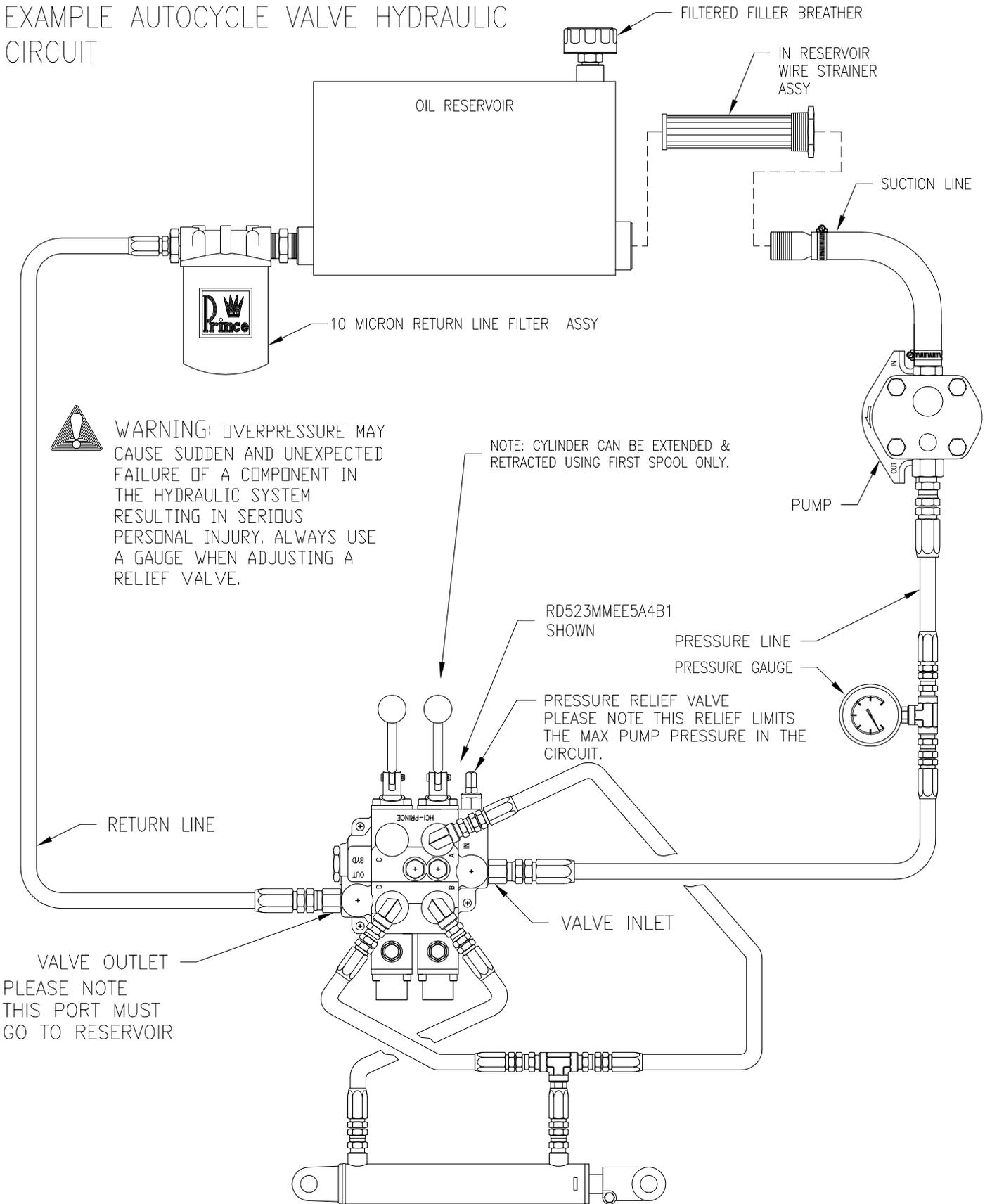
NOTE: THIS VALVE IS FACTORY TESTED AND SET. NO ADJUSTING SHOULD BE NECESSARY. IN A NEW INSTALLATION MAKE SURE ALL AIR IS OUT OF LINES BEFORE MAKING ADJUSTMENTS. CYCLE CYLINDER UNTIL OPERATION STABILIZES. DO NOT ADJUST IMMEDIATELY UPON INSTALLATION.
