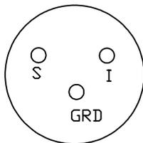
Switch On: Volts from I go GRD should be approx battery voltage.
