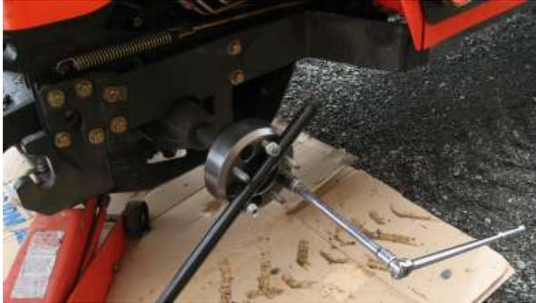
H. Get your socket & add Loctite to the studs on the spacer. Install the rim/wheel & now use the new Lock Washer & nuts from the spacer, making sure they are flip to the proper end. Torque the nuts to 110 ft. lbs for the rim in the same 3 steps as above.
