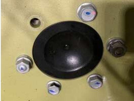
F. The factory bolts treads are 14mmx1.5 tread, We have supplied new Lug bolt 14mmx1.5 use these to install the spacer to the axle
