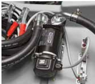
12 volt transfer pump delivers fuel at 10 gallons per minute.
