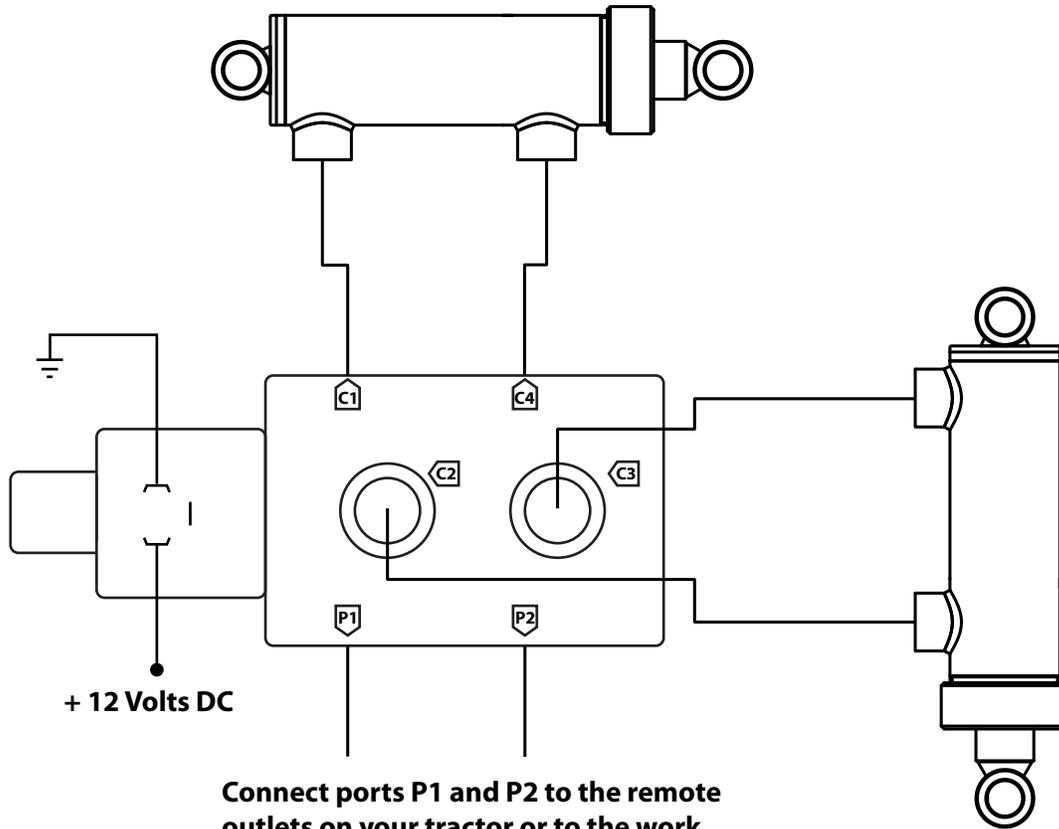
Connect ports P1 and P2 to the remote outlets on your tractor or to the work ports of a double acting valve, whichever applies.
