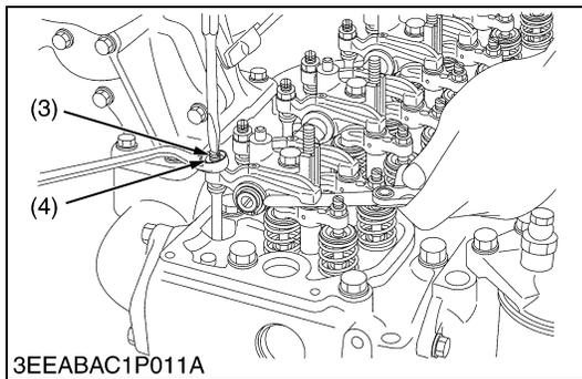
**Checking Valve Clearance**
