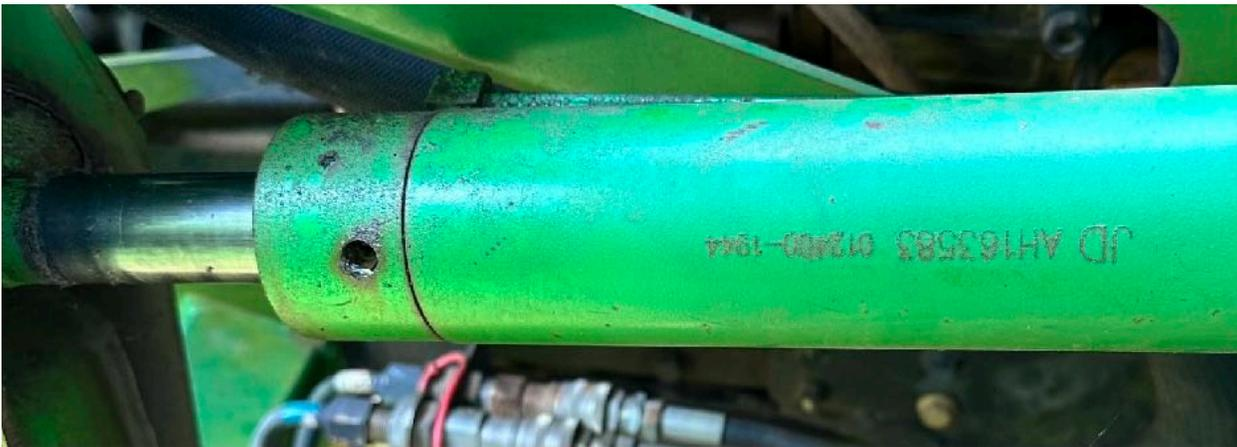
The cylinder wire appears to be a staple, lift the end up to enable movement:
