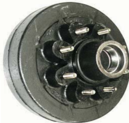
8 Lug hub Drum with 1 3/4" inner brg # 25580 & 1 1/4" outer brg
