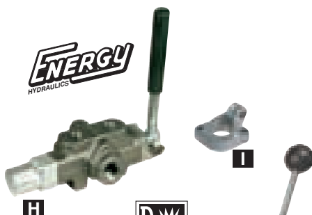
H) Max. continuous pressure: 2,500 PSI • Relief set at 2,000 PSI • Max. continuous flow: 20 GPM • Work Ports: 1/2" NPT • Inlet/Outlet Ports: 3/4" NPT 1242296 – Wt. 9.0 lbs. .... 129 99
