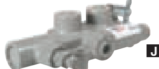
J) Max. continuous pressure: 2,750 PSI • Relief set at 2,250 PSI • Max. continuous flow: 25 GPM • Kick-off pressure adjustable from 1,000 to 3,000 PSI • Work ports: 1/2" NPT • Inlet/Outlet ports: 3/4" NPT 8107203 – Wt. 10.2 lbs. .... 119 99
