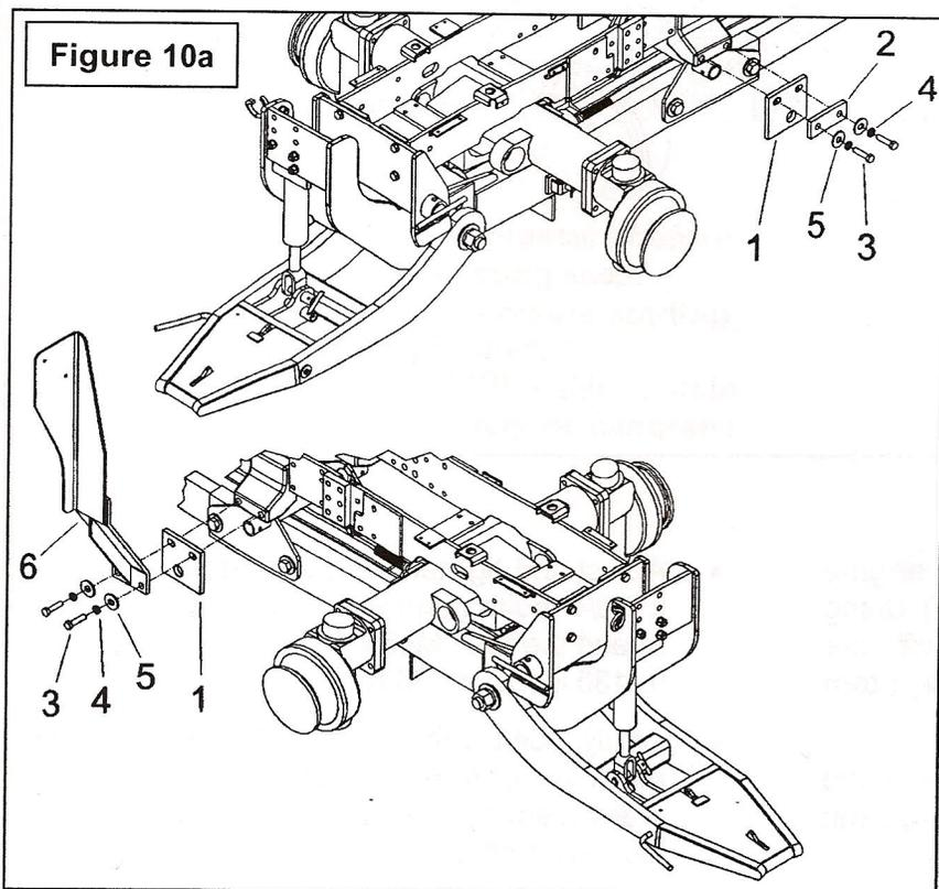
**NOTE:** Position the round hole of the installation plates (Fig. 10a and 10b, item 1) towards the rear of the tractor.
