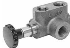
• New PARKER Model HM-Series. For snow plows, loaders, winches and similar equipment. Use with standard 4 way, 3 position valves to provide a float or free wheeling position. 10 GPM, max. 2000 PSI, chrome plated pressure balanced spool. Size 6" x 3" x 2 1/4". Shpg. 5 lbs.
