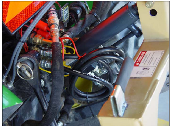
Hydraulic Top-Link in fully raised and retracted position.
