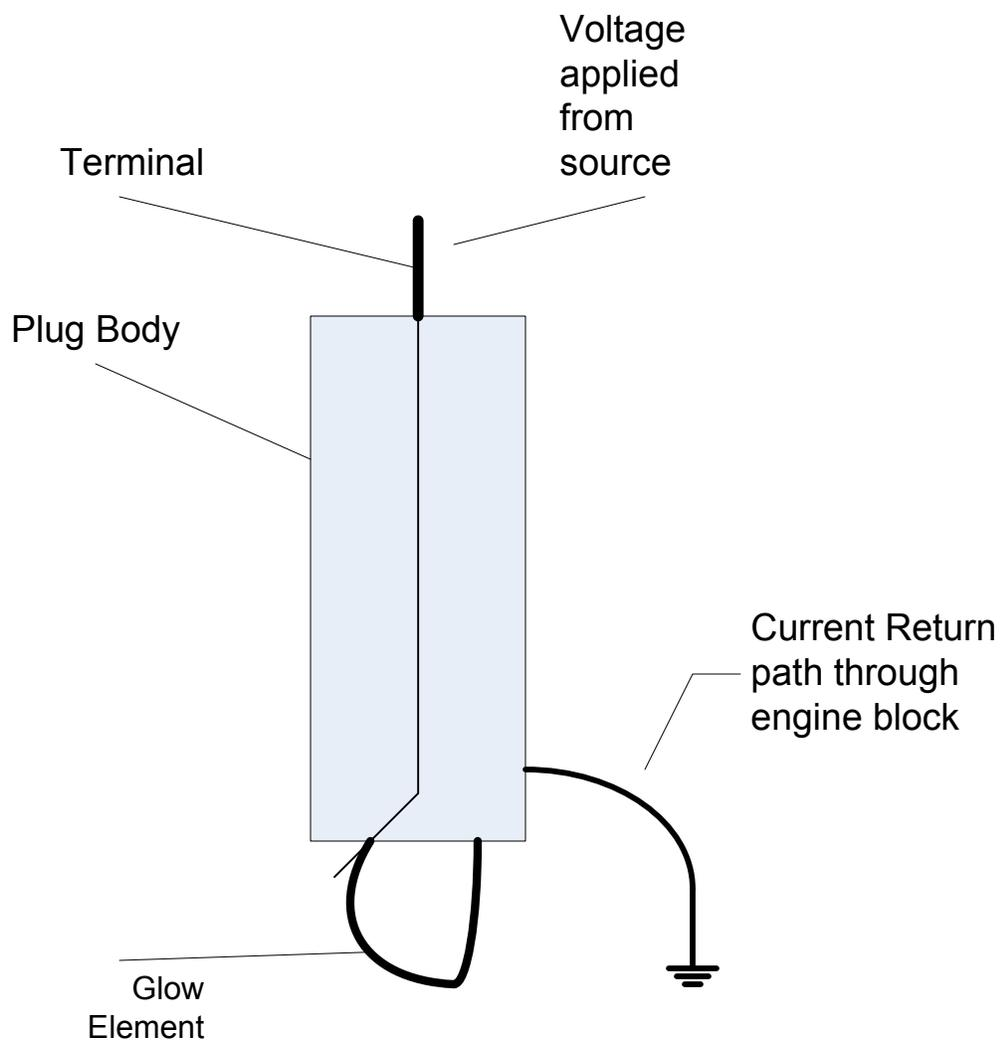
There is no way that this plug can be connected in series with other plugs with only one terminal to connect to. If this is the case, the plugs must be connected in parallel.
