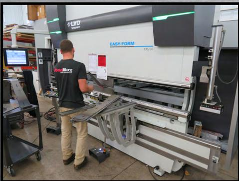
◀ 150-ton press brake with EFL(easy form Laser) laser measuring for precise bends.
