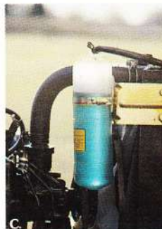
A. Thermo-start. B. Heavy-duty air cleaner. C. Coolant recovery system. D. 4-way flashing lights on turn signals. E. Position control. Draft Control F. Full flow hydraulic oil filter. G. Foot operated differential lock.
